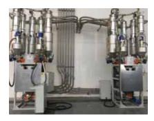
Example of centralized dosing system with a production capacity of 2000 kg / h. This application is able to feed 10 extrusion lines with the possibility of setting a different recipe for each line, choosing from 8 virgin materials.
